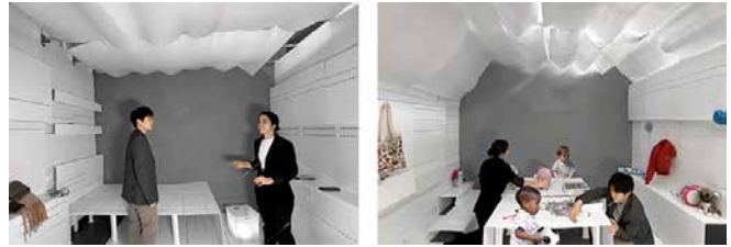
Fig. 2. Our rapid-prototyped, 80 sq ft robot-room: two physical configurations, same view, supporting bedtime and playtime. The prototype is made of corrugated plastic sheets, laser-cut, suspended inside an extruded-aluminum frame.
